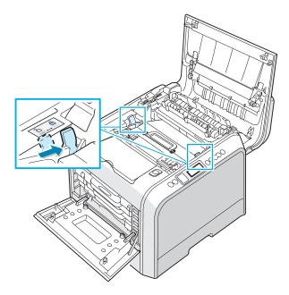
13 After making sure that the left cover is open, close the top cover. Make sure that it is securely latched.
